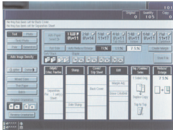
The 9002/10512 Control Panel enables quick access to all of the advanced capabilities.
