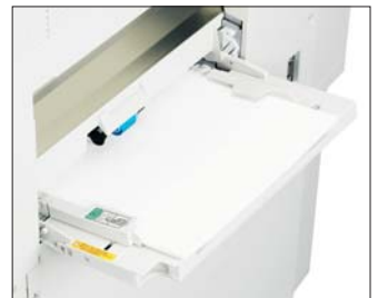
The 100-Sheet Bypass Tray accepts paper sizes up to 12" x 18".
